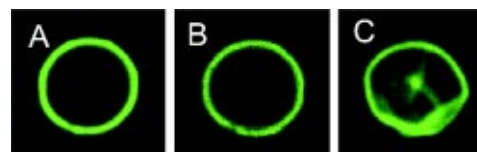
FIG. 3. Typical confocal images of MF capsules (radius R_0 = 2 \mu\text{m} ) obtained for different stages of deformation: (a) \epsilon = 0 , (b) \epsilon = 0.2 , and (c) \epsilon = 0.5 .
