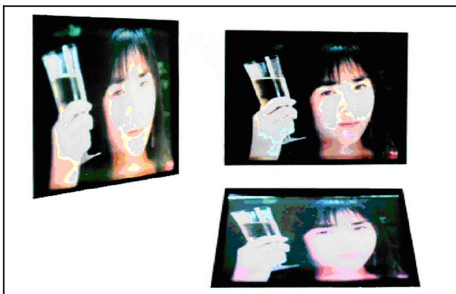
Figure 1. Casio's 2.5-inch diagonal 832×230 active matrix TLAF prototype. The drive voltage is \pm 2.5 V; time to scan one line, 60 \mu s; and contrast ratio over 300. The upper right is a front view. The other images show no grey scale inversion nor colour change even when the viewing angle is as in the lower right [6]. Courtesy T.Yoshida: tyoshida@drd.hlb.casio.co.jp
